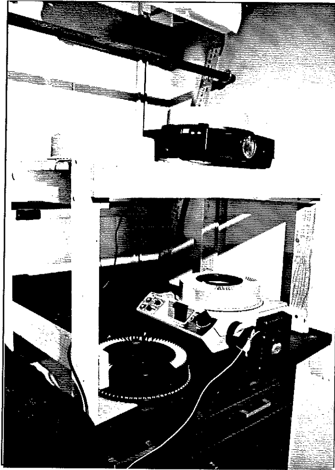
Figure 8. Slide projectors used in the laboratory BFOV experiment showing the tachistoscope shutter open on the stimulus projector.
