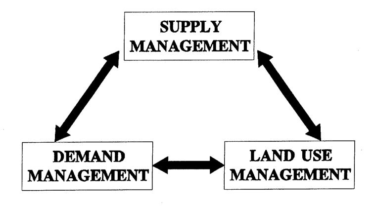
Figure 1. Elements of a typical congestion management program.
