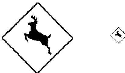
Figure 60. Scaled PICT images of Deer Crossing sign as sized at 441.9 and 103.6 meters from sign
