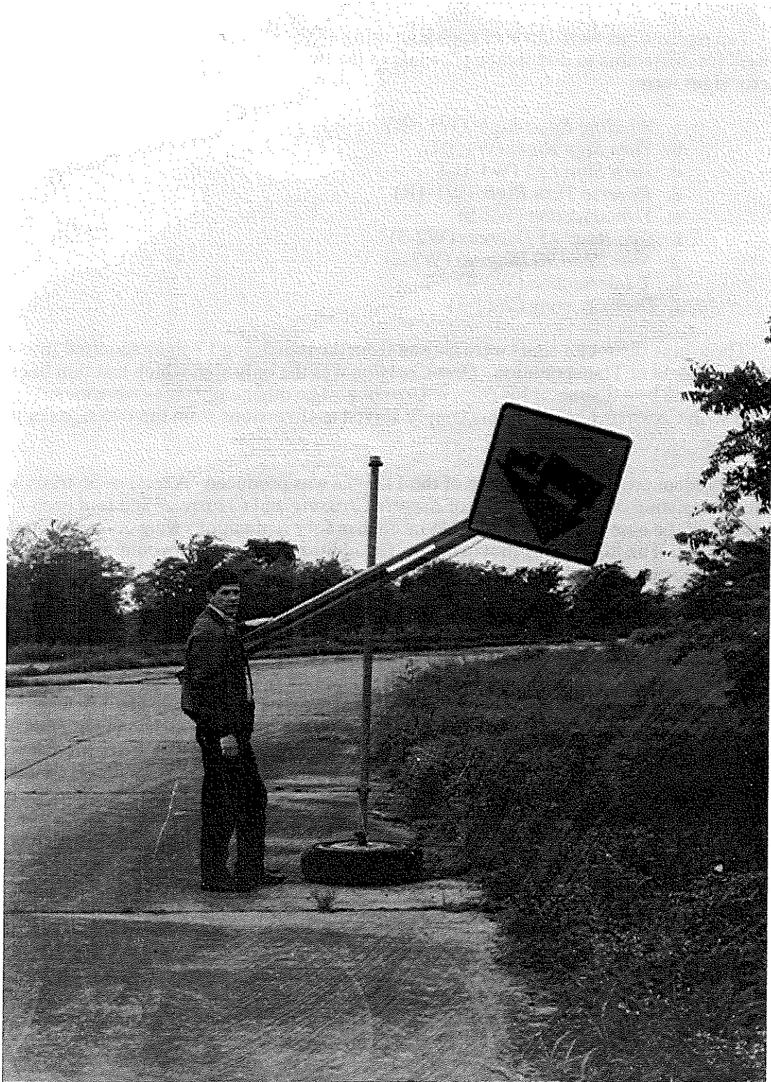
Figure 7. Operation of quick-change mounting pole for signs
